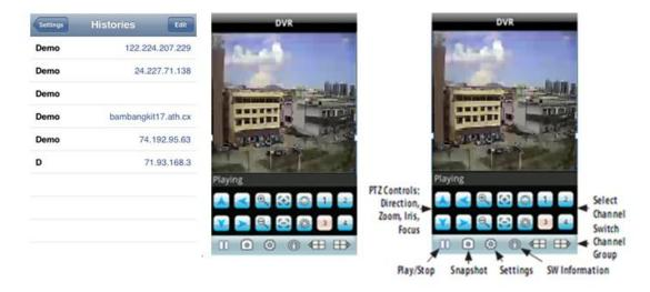
To view a particular camera, tap the Select Channel button for the camera channel. If you are connected to an 8- and 16-channel system and the channel button is not shown, tap a Switch
